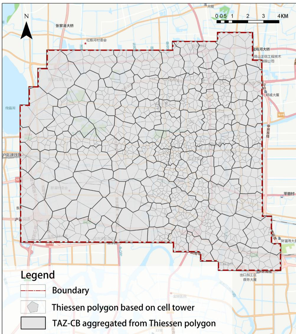
**Figure 2.** Cell tower coverage and TAZ-CB diagram
