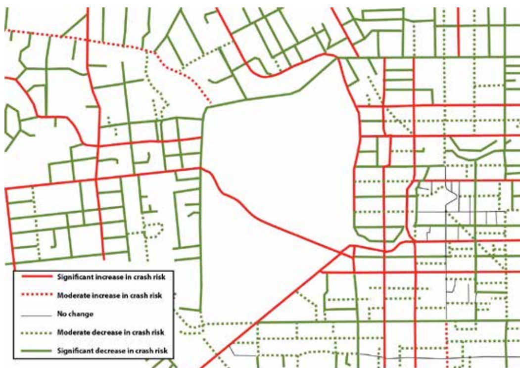
Figure 2: Changes in bicycle–motor vehicle crash probability for a portion of Christchurch due to spatial characteristics present in the road environment
