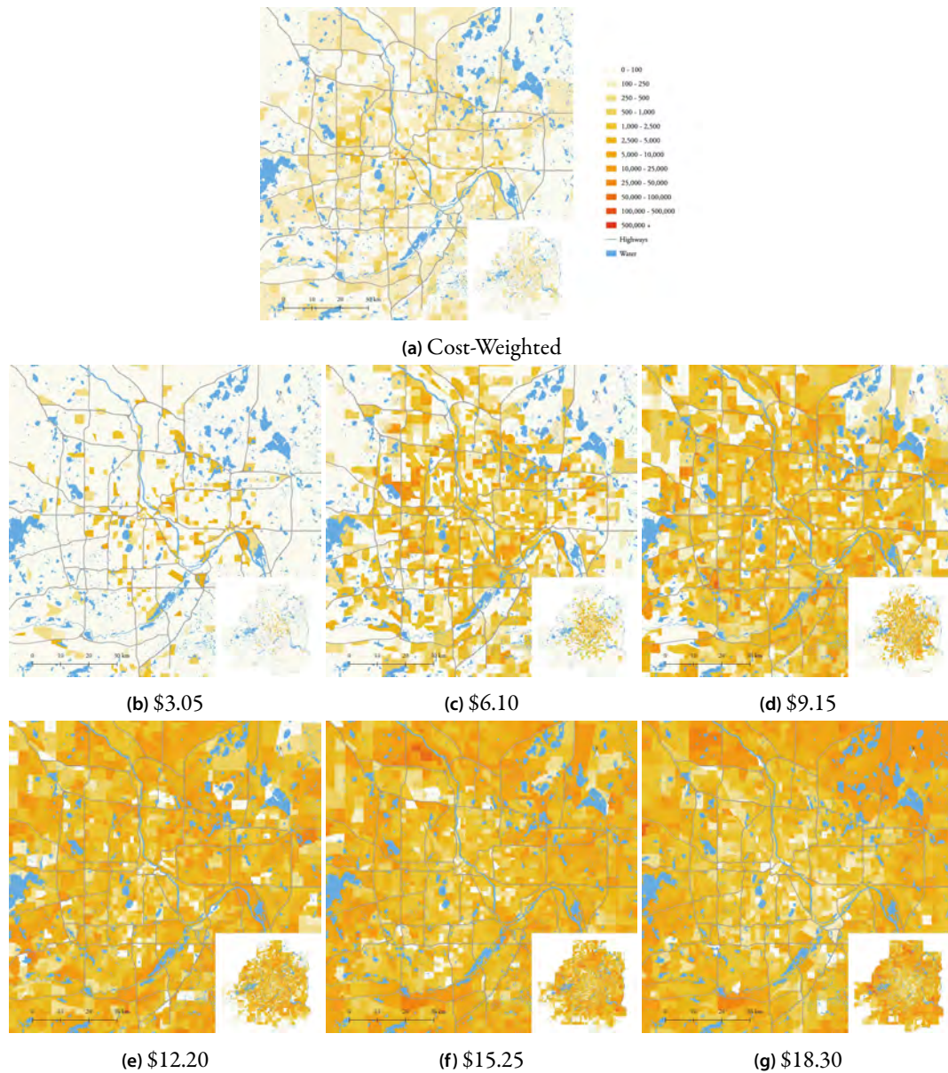
Figure 12: Internal Cost Accessibility Loss Using the Shortest Travel Time Path Compared with the Lowest Internal Cost Path, Based on the Cost-Weighted Results and with the Internal Cost Threshold [$3.05 to $18.30] (Lowest Internal Cost Path - Shortest Travel Time Path)
