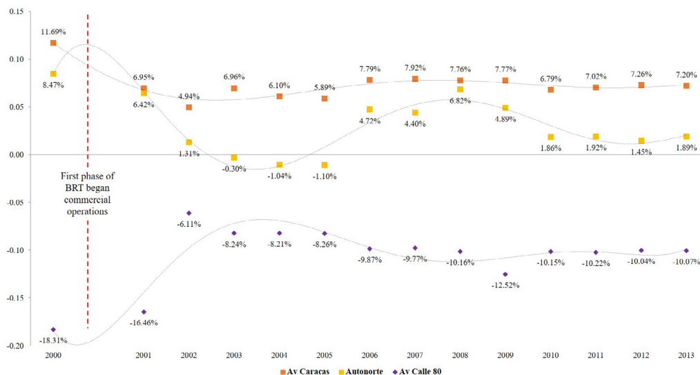
Figure 3. Estimated average effect of BRT on built-up area change (percentages) over time by BRT corridor, Bogotá, Colombia
