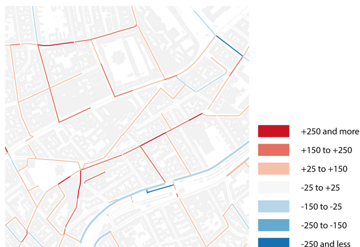
Figure 4. Change of vehicles at peak hour at street level for a selected inner-city street and surrounding streets: comparison between scenario 1 and reference scenario
