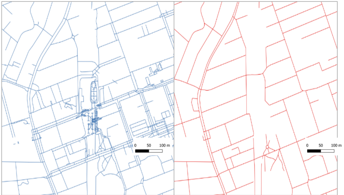
Figure 3. Two maps of Chatswood, a commercial center in Sydney, showing the difference in detail between OSM (left) and Geoscape (right) pedestrian network data; additional detail is mostly pedestrian paths through shopping malls, parks, and a train station, which are significant for accurate routing.
