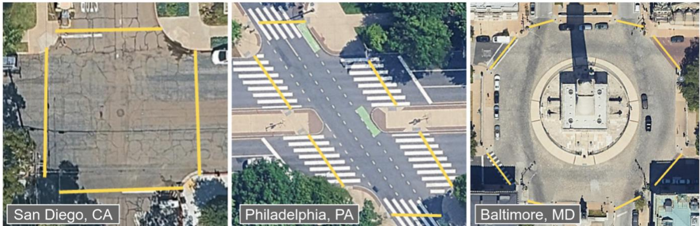
Figure 9. Automatically generated crossing distances at intersections of varying complexity in San Diego (left), Philadelphia (center), and Baltimore (right), including both marked and unmarked crossings
