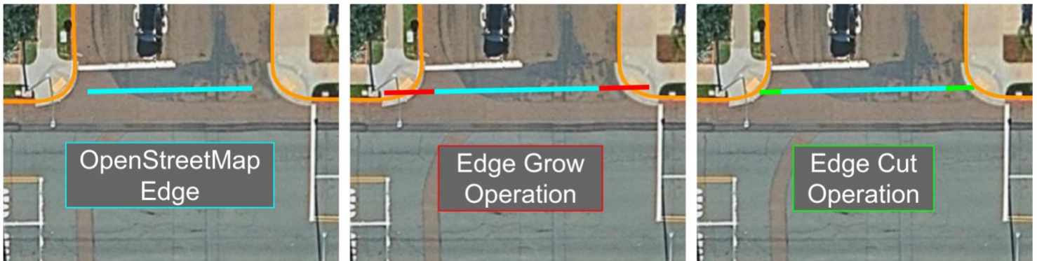
Figure 7. Grow-cut algorithm sequence, in which the crosswalk edge from OpenStreetMap (left) is first grown by a magnification factor (center), and then cut based on the boundary of the non-drivable space segmentation (right)
